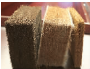
左边是山棕,中间是纤维胶黏合的椰棕,右边是化工胶黏合的椰棕
